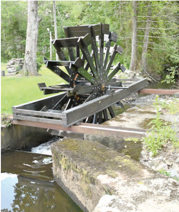
The water wheel located at the Wolcott Lions Fairgrounds is back in working condition once again. The original wheel was installed a few years ago by Lion George Phelan with the help of Wolcott High students in the Industrial Arts Department. A severe rain storm destroyed the original wheel when water levels and volume in the stream it straddles, was too much for the wheel to handle.
